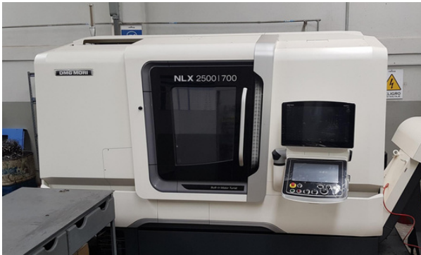
DMG MORI NLX 2500 / 700 with live tooling
